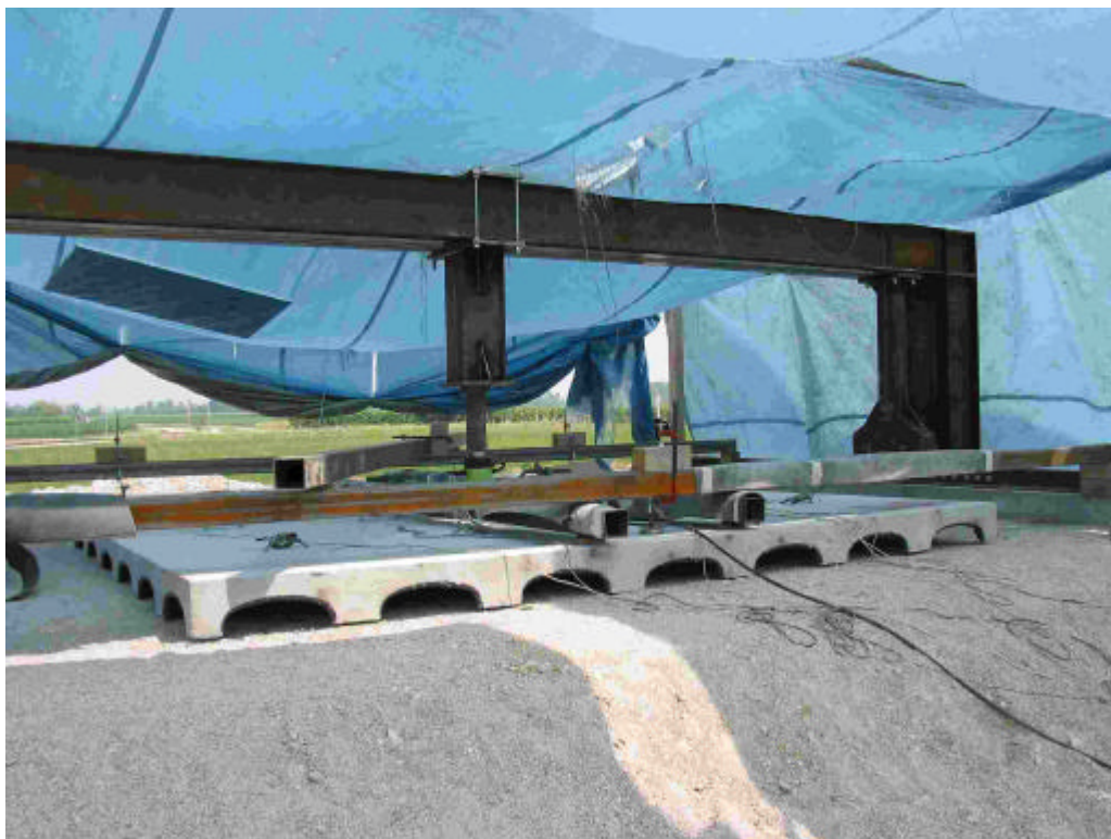
Fig. D.22 Concrete test n°11 on gravel subgrade
