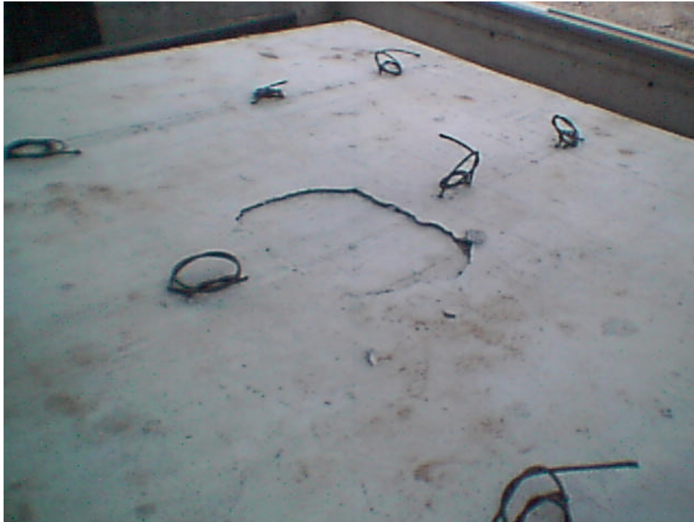
Fig. D.21 Punching Crack on the concrete test n°7
