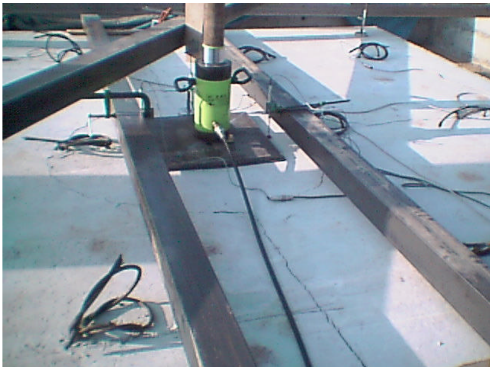
Fig. D.14 Crack line and instruments detail on the concrete test n°4
